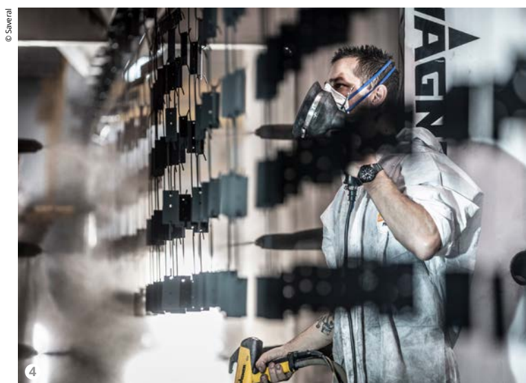
Figures 4 and 5: The line for coating parts with a maximum size of H 1800 x W 4000 x D 1000 mm, featuring a Wagner quick colour change booth.
