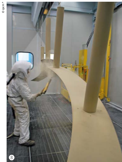
Figure 8: The line is able to handle workpieces with maximum dimensions of H 2500 x W 6000 x D 2000 mm.
